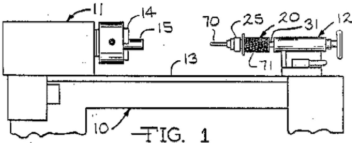
This tool can be used in its simplest application as a rather long tailstock drill chuck to drill a workpiece mounted in the lathe. Because the EZ-Tapper cannot rotate while in its rightmost position (where it is held both by its spring loading and by the pressure of the drilling operation), it does not rotate during drilling.
