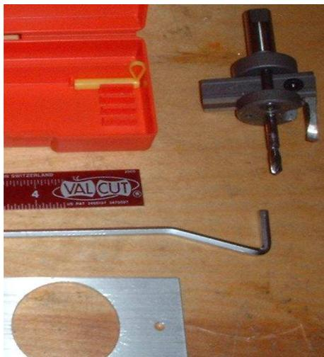
this one. It cuts smoothly and cleanly in a low horsepower, non-rigid machine like a mill-drill. It will be used for making mounting holes for stepper motors and tube sockets. It is capable of making interrupted cuts and overlapping holes.
