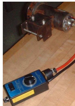
Murray's Auto Parts. The motor is a 2-1/4HP 120Volt DC, and he got a Harbour Freight variable speed AC controller and added a rectifier bridge to control the DC motor with 120Volts AC, controllable from about 25 to 3000 RPM. Works slick for very little cost, and is very powerful. He thinks he will install it on a drill press.
