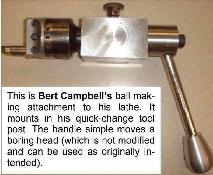
This is **Bert Campbell's** ball making attachment to his lathe. It mounts in his quick-change tool post. The handle simple moves a boring head (which is not modified and can be used as originally intended).
