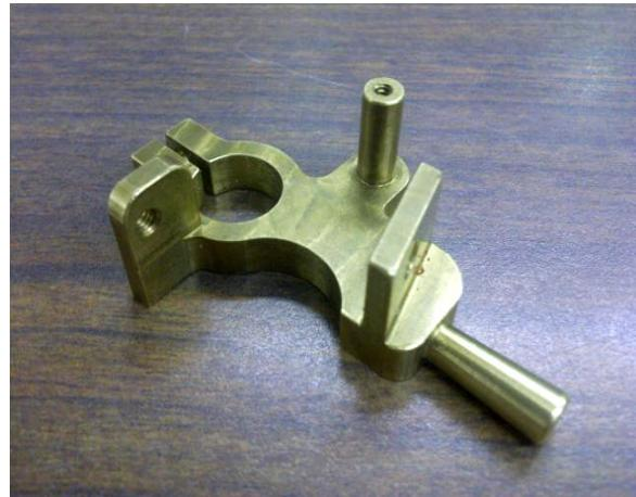
Here is another view, oriented upright. The top stud is a lever used to vary the ignition timing while running:
