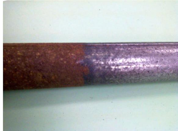
Don notes that the process removes ‘red rust’ but leaves behind a thin coating of ‘black rust’ which is easily wiped away. The part must be protected quickly from flash rusting, either by oiling or by a protective finish. This technique is particularly useful for parts with difficult shapes, like fuel tanks or parts with internal features not easily scrubbed.
