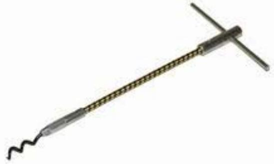
Brian identified it as a packing-puller, used to remove packed shaft sealing material from centrifugal pump housings.
