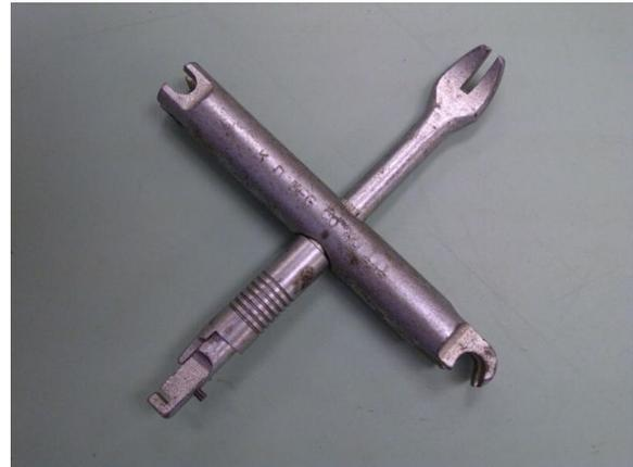
Apparently we have all become spoiled by modern no-maintenance electronic ignitions because nobody had a quick answer. It turned out to be an ignition ‘multi-tool’ used to open distributor caps for access to the breaker, rotor and capacitor ... remember those? It also appears to have a spark plug gapping feature and perhaps other uses lost to time.
