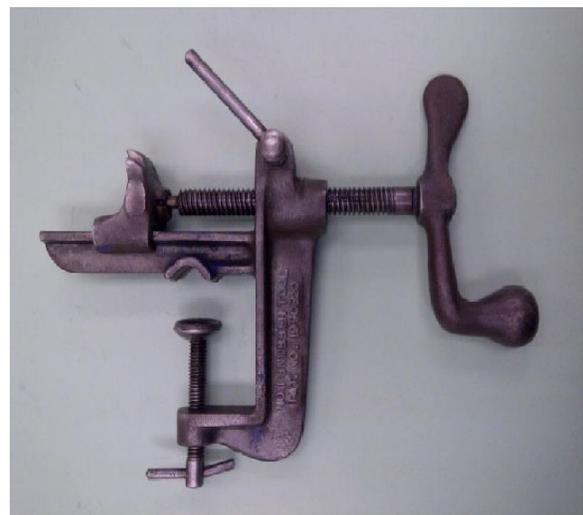
The lever at the top operated a knurled cam (apparently intended to grip something being stretched or tightened by the screw), and the lower screw allows the device to be clamped to a post or bench. The cast iron frame is marked “Hose Stay Put Tool Co., Denver, Colo.” –
