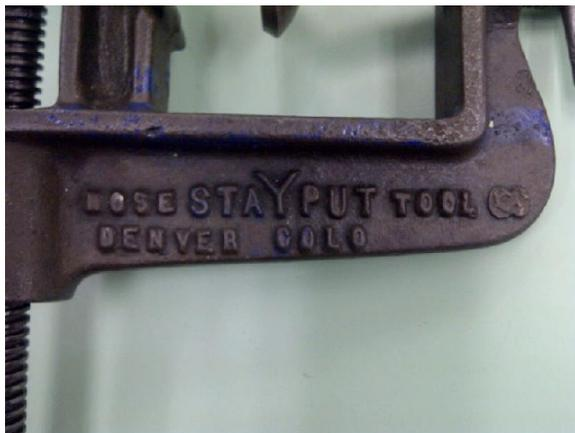
A patent number was marked on the opposite side and some post-meeting research revealed that this device was patented in February, 1935 “for the usual purpose of securing one hose section to another or for the attachment of a coupling-member at the end of a hose” using ordinary wire. The wire is looped around the hose, the ends are secured by the knurled cam, the wire is stretched tight by the screw, and the wire ends are then twisted, released from the cam and trimmed to length.
