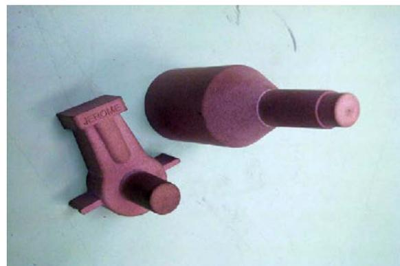
The cone in the upper picture is simply the casting sprue, removed when cool. The engine runs on diesel fuel (or some similar concoction) and lacks a traditional spark or glow plug. Ron Peters noted that compression alone *will* ignite the fuel even in a cold engine if a bit of ether is added to the starting charge. Here is a link to a YouTube video of such an engine running, quite nicely –
