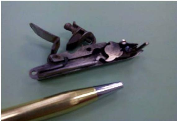
Jim is a metallurgist, retired in '05 from Rolled Alloys, Inc. (formerly in Detroit, now located in Temperance, Michigan - [www.rolledalloys.com](http://www.rolledalloys.com) ). Jim's project was made using a jeweler's lathe, files, and a cold formed spring which he tempered himself –
