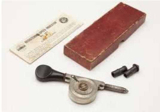
Note the rubber tips on the right side of the picture. Ken's have hardened and cracked and no longer work well. He is looking for a suitable substitute or source of replacements. Several members suggested simply attaching a pencil eraser (the 'slip on' ones so common when pencils were still used) and then using a sander to reshape their chisel shaped ends to a point, or ball, or whatever is needed.
