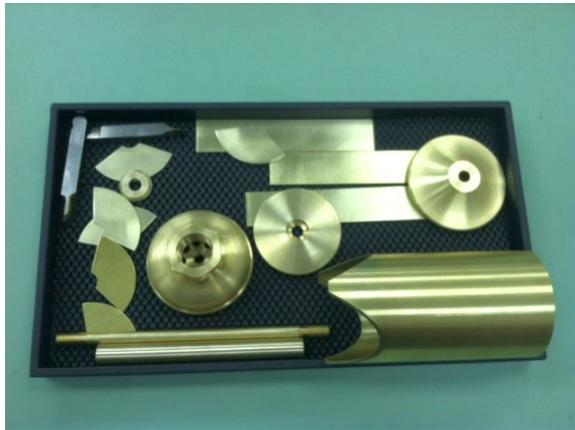
The outer body is 3" diameter with a 0.875" wall. A disk at the bottom forces air along the sides of the chamber wall for more effective flow past the slots:
